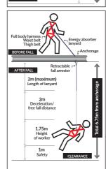
used together to create one attachment point. The opposite end of the lanyard is to be connected to the anchorage connector. Always use structural anchors provided as an anchoring point if possible. Ensure that any anchoring point used have a resistance of 12KN or more and is suitable under EN795.
